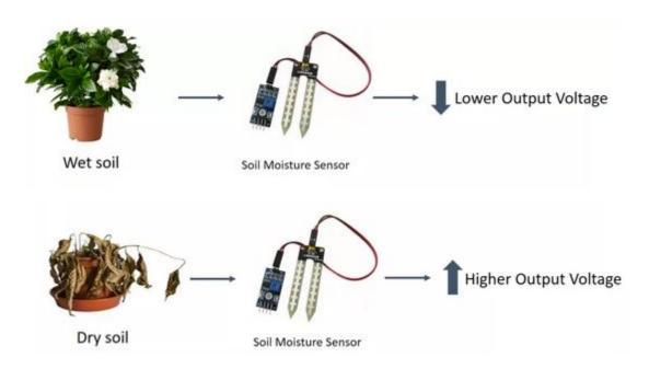
The output can be a digital signal (D0) LOW or HIGH, depending on the water content. If the soil humidity exceeds a certain predefined threshold value, the modules outputs LOW, otherwise it outputs HIGH. The threshold value for the digital signal can be adjusted using the on-board potentiometer. The output can be a analog signal and so you'll get a value between 0 and 1023.
